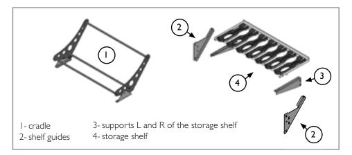
I) Place the storage shelf supports on the interior walls at the back of the cabinet.
