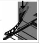
**4**) Position the cradle on the **unloaded** sliding shelf and screw on.
