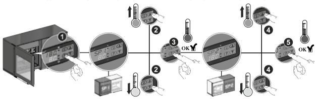
I Press the P key. the message "SPI" will appear. You can now set the temperature of the left-hand compartment.
