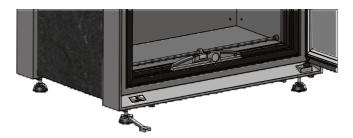
Using a 19 mm open-ended spanner and spirit level, set the feet of your cabinet so thatit is completely stable.
