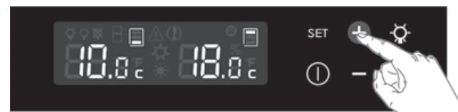
2 Press the **+** or **-** keys to set the desired temperature.
