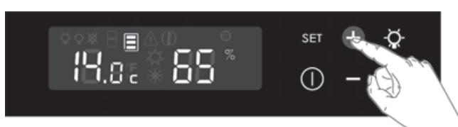
2 Press the **+** or **-** keys to set the desired temperature.
