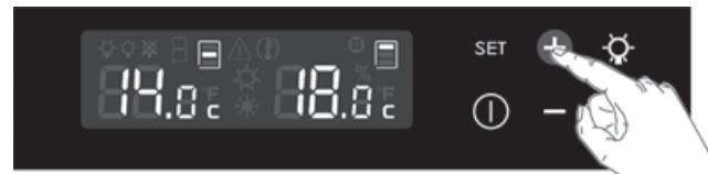
2 Press the **+** or **-** keys to set the desired temperature in the maturing compartment.
