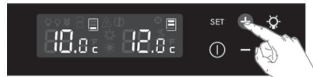
2 Press the **+** or **-** keys to set the desired temperature in the chilling compartment.
