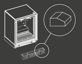
When the cabinet is installed with the hexagonal pillars to be elevated, you must adapt the shape of the separators. This is important in order to correctly guide the air flows downwards and therefore to the ventilation grid (incoming or outgoing).
